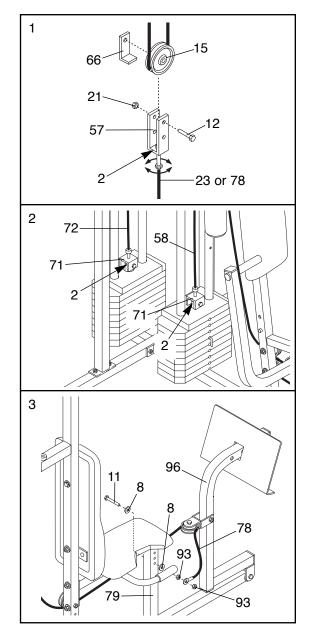
If a cable tends to slip off the pulleys often, it may have become twisted. Remove the cable and re-install it.
